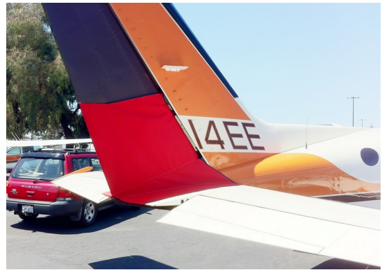
Cessna 414 Rudder Openings Cover (bird barrier)
