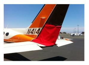
Cessna 414 Rudder Openings Cover (bird barrier)
