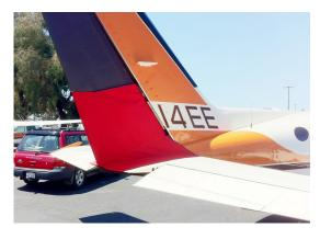
Cessna 414 Rudder Openings Cover (bird barrier)
