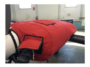
Cessna 402 Insulated Engine Cover with Heater
