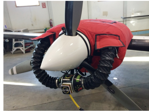
Cessna 402 Insulated Engine Cover with Heater
