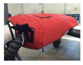
Cessna 402 Insulated Engine Cover with Heater
