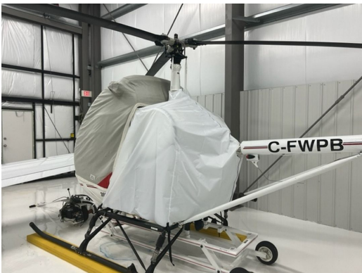
Schweizer 300C Engine Cover, test fit cover
