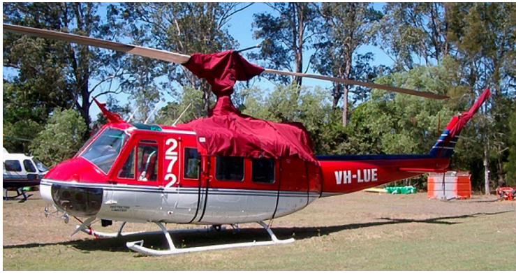
Bell 204/205 Engine/Mid-Cabin Cover, Main & Tail Rotor Covers
