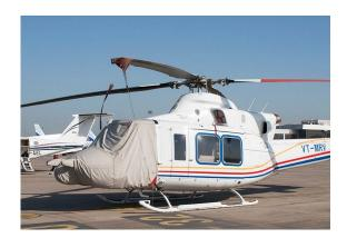
Bell 412 Forward Cabin/Nose, Insulated Engine, Tailboom, Rotor Hub & Blade Covers
