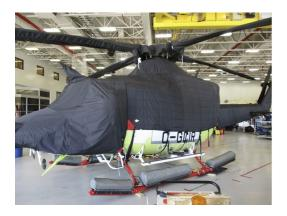
Bell 412 Forward Cabin/Nose, Insulated Engine, Tailboom, Rotor Hub & Blade Covers
