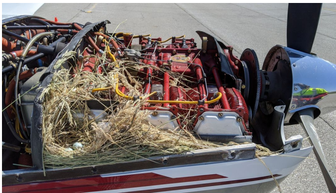
ENGINE PLUGS PREVENT BIRD NEST FOD. Piper Saratoga Engine Cowling Bird's Nest Engine and Oil Cooler Inlet Plugs
