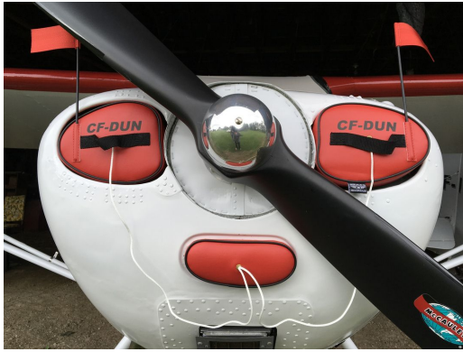
Aeronca 11AC Engine Inlet Plugs
